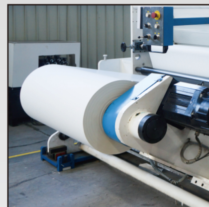
Unwinding (The material tension is controlled by a closed loop of the brake or servo motor.)
