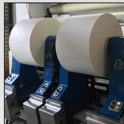
Winding (The independent winding station realizes adjustable tension for each roll.)
