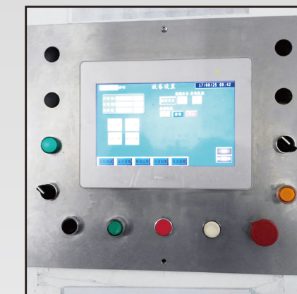
Simple operation (A human-machine interactive interface that displays all data information of the machine.)
