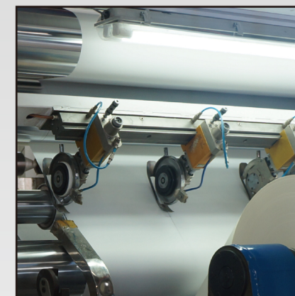
Slitter (Quickly change orders with the automatic cutting tool setting system.)
