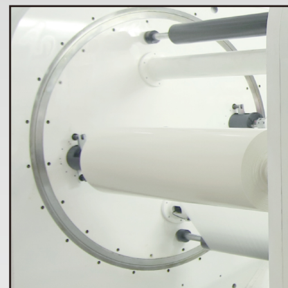
Unwinding (The unwinding with shear-plate is unstopped which the structure is stable and reliable. With closed-loop tension control and automatic winding diameter calculation, unmanned roll change is realized. )
